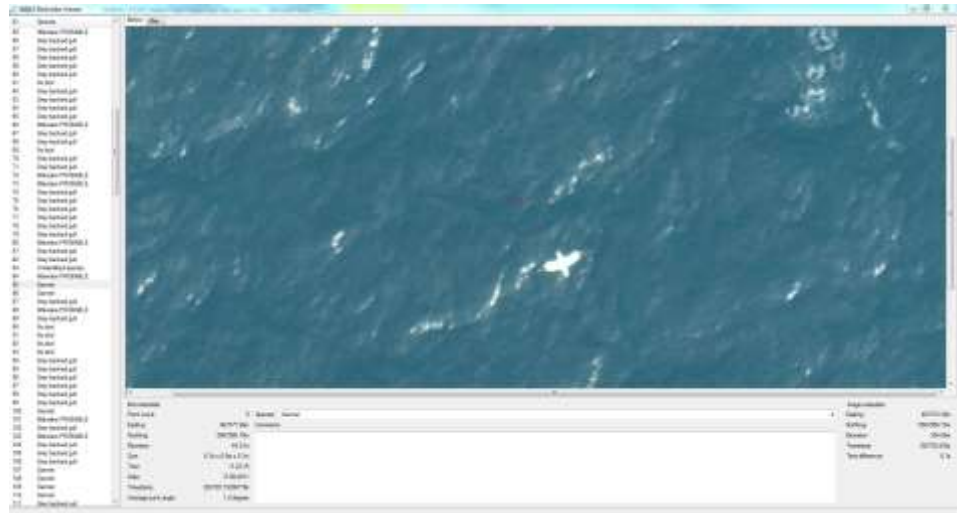
Figure 4.1: LiDAR Cluster and associated "before" picture showing bird classified as Gannet flying at 1.31 m (44.31 m elevation above ETRS89)
